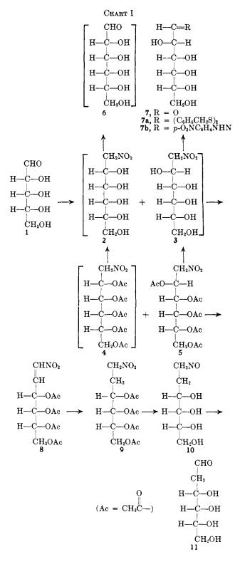
acetylated in the same manner and the resulting crude hexitol (10), without further purification, was subjected to the Nef reaction giving 2-deoxy-D-allose (11) in 38% yield based on the hexene (8) demonstrating the superiority of this method for converting an acetylated nitro alcohol to the corresponding aldose.
